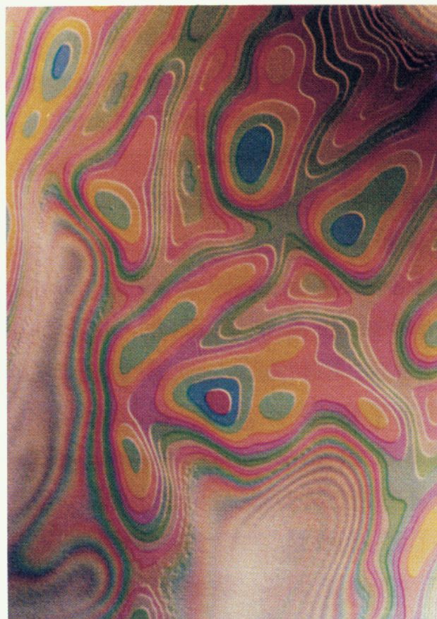
Figure 12. Nomarski micrograph of a PSD/PMMA copolymer sample annealed at 170 °C for 24 h. The color bands at the edge of the sample are clearly demarcated by bright white lines. The full, long dimension of the micrograph is 280 \mu\text{m} .
