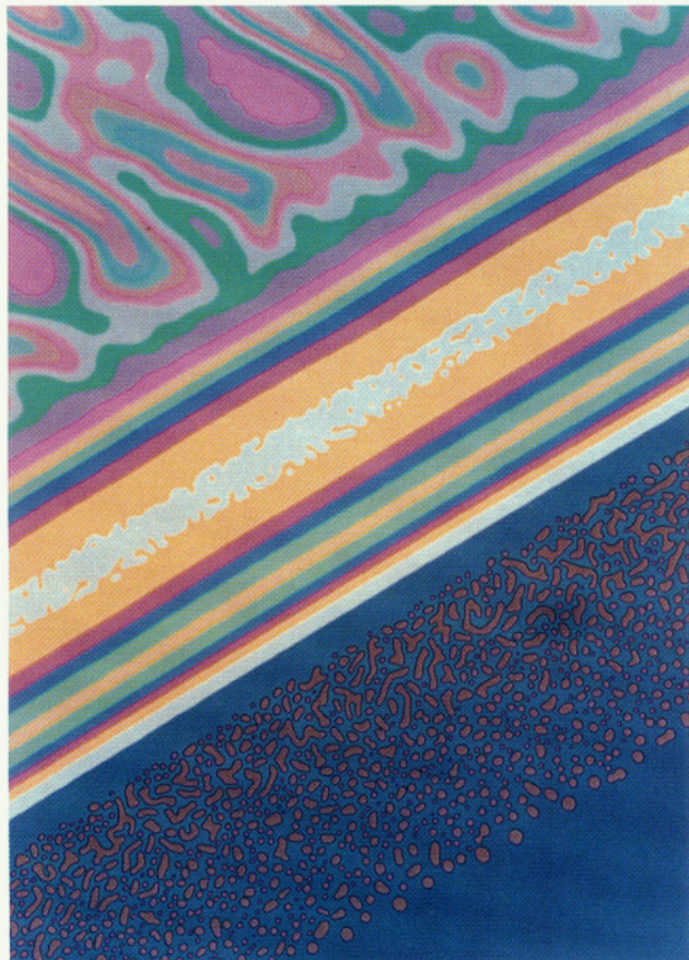
Figure 11. Interference colors observed at the edge of a PSD/PMMA copolymer sample annealed at 170 °C for 24 h. The full, long dimension of the micrograph shown is 280 \mu\text{m} . The orientation of micrograph is the same as that in Figure 10.
